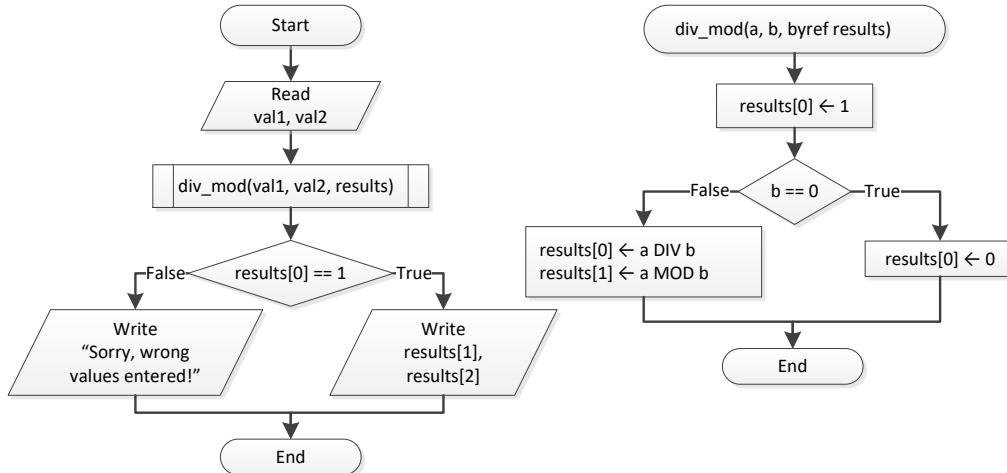
**Notice:** Flowcharts are a loose method of representing an algorithm. Thus, you can represent a pass by reference using the keyword `byref`, which clearly denotes what it actually does.
